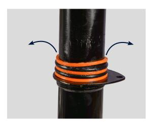
**4.** Remove and discard the existing backup rings (3x) and O-rings (2x).
