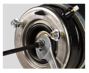
Remove the nut at the top of the strut: Insert a M8 Allen key into the pin and hold whilst unscrewing the nut using a M24 spanner. Lift-off the washer freed by removal of the nut. Then clamp the strut in a vice at the lower end. Use protective jaws in order to avoid damaging the component.
