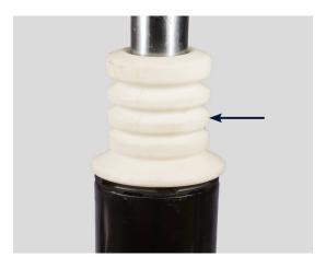
7. Place the bump stop from your kit over the neck of the shock absorber and onto the seat.
