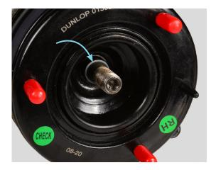
Apply silicone-based lubricant to the O-rings and insert 2 O-rings and 2 backup rings from your kit into the annular cavity between the shock absorber and the top mount of the air spring bag. Insert parts in the order (from bottom) O-ring > backup ring > O-ring > backup ring as indicated.
