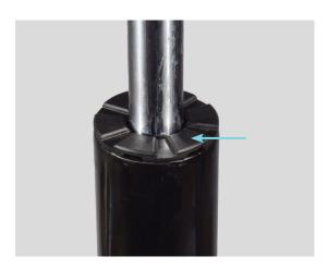
6. Place the bump stop lower seat disc from your kit onto the "shoulder" at the upper end of the shock absorber tube, with "teeth" facing upwards as shown.
