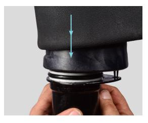
Place the new air spring bag from your kit onto the shock absorber assembly so that the pin at the base of the piston is inserted into the hole in the piston seat.
