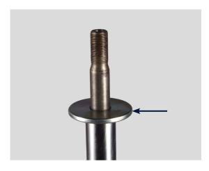
Place the reaction washer from your kit onto the "shoulder" at the upper end of the shock absorber.
