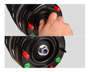
12. Install the M16 nyloc nut from your kit: Insert a M8 Allen key into the pin and hold whilst tightening the nut. Ideally use an open-ended torque wrench with a 24 mm fitting and tighten to torque 75 Nm (55lb.ft), otherwise hand-tighten with a 24 mm spanner.
