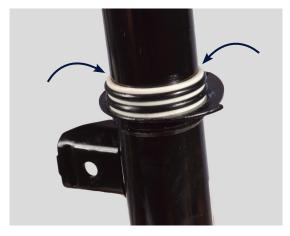
**5.** Place the backup rings (3x) and O-rings (62.0x5.0, 2x) from your kit over the shaft at the top and down onto the piston seat in the silicone-based lubricant to the O-rings.
