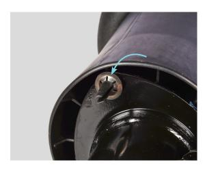
2. Pry-off and discard the star lock fastener that secures the pin at the underside of the air spiring module piston.
