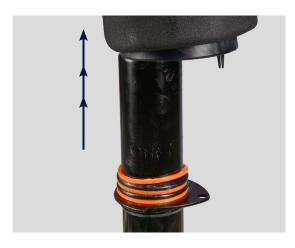
**3.** Gently tap the piston from below using a soft-face mallet in order to lift the piston from it internal seals. Lift-off the air spring bag from the shock absorber.
