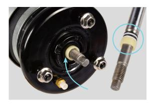
Apply silicone-based lubricant to the O-rings and insert 2 O-rings, 2 backup rings and the plastic guide ring from your kit into the annular cavity between the shock absorber and the top mount of the air spring bag. Insert parts in the order (from bottom) O-ring > backup ring > O-ring > backup ring > plastic guide ring as indicated.
