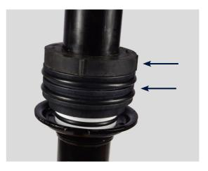
Now place the plastic piston at the end of the shock absorber tube with the contraction facing upwards as shown. Then place the rubber washer over the plastic piston.
