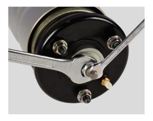
Remove the nut at the top of the strut: Insert a M8 Allen key into the pin and hold whilst unscrewing the nut using a M21 spanner. Lift-off the washer freed by removal of the nut. Then clamp the strut in a vice at the lower end. Use protective jaws in order to avoid damaging the component.
