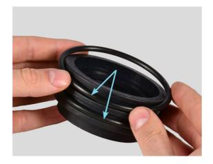
Replace the large O-rings on the plastic guide piston before placing it on the shock absorber.
