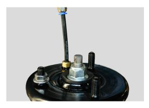
Clamp the strut in a vice and attach an air line. While inflating the air spring with pressure to around 3.5 bar (50.8psi) at the same time pull the lower piston over the sealing ring. As soon as the air spring closes, it moves to the end position (see picture on the right).
