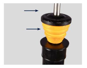
Over the top end sleeve place the new rubber buffer of the kit and your old metal disk to hold the rubber buffer.
