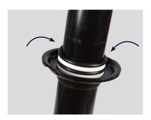
5. Place the new backup rings (2x) and O-rings (2x) from your kit over the shaft at the top and down onto the piston seat in the silicone-based lubricant to the O-rings
