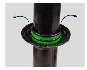
Remove and discard the existing backup rings (2x) and O-rings (2x).
