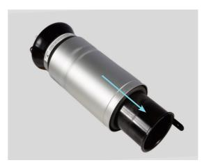
Before placing the air spring on the shock absorber, pull out the lower piston.
