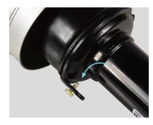
2 . Remove the plastic locking pin at the underside of the  $\,$  air spiring module piston.
