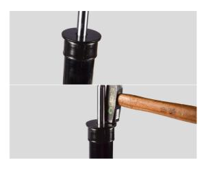
8. Slide your old top end sleeve onto the top end of the shock absorber and tap it with a hammer to prevent it from slipping.
