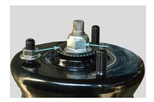
13. Insert the upper washer from your kit in the orientation shown. Then install the M12 nyloc nut from your kit: Insert a M8 Allen key into the pin and hold whilst tightening the nut. Ideally use an open-ended torque wrench with a 21 mm fitting and tighten to torque 75 Nm (55lb.ft), otherwise hand-tighten with a 21 mm spanner.
