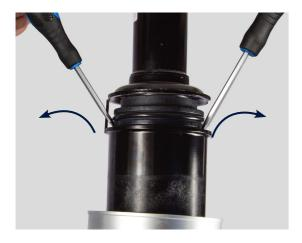
**3.** Gently pry out the piston from below as shown in the picture in order to lift the piston from its internal seals. Lift-off the air spring bag from the shock absorber.
